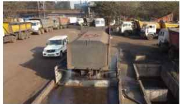
Mechanized wheel washing system
